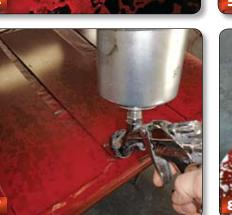
I cut several pieces of aluminum blanks commonly used in the sign industry—8-inches by 24- inches, scuffed them with a red Scotch-Brite pad to establish a tooth to the surface, and applied a black automotive base coat with a spray gun.
